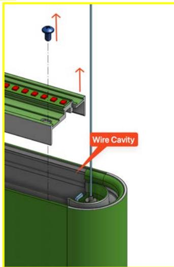
9. Remove power cord break away tab to feed power cord into the wire cavity.
